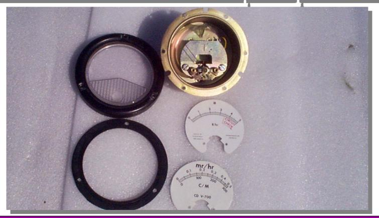
NOTE: Use the procedure in FEMA Repair and Maintenance Manual for Radiological Instruments, Volume 10, Appendix F, Page F-35, METERS.
