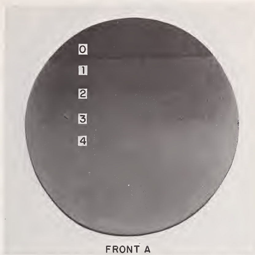
Fig. C.5a. SOT topograph of A surface damage (front), reduction in contrast after each step represents a direct measure of distribution of damage below surface.
