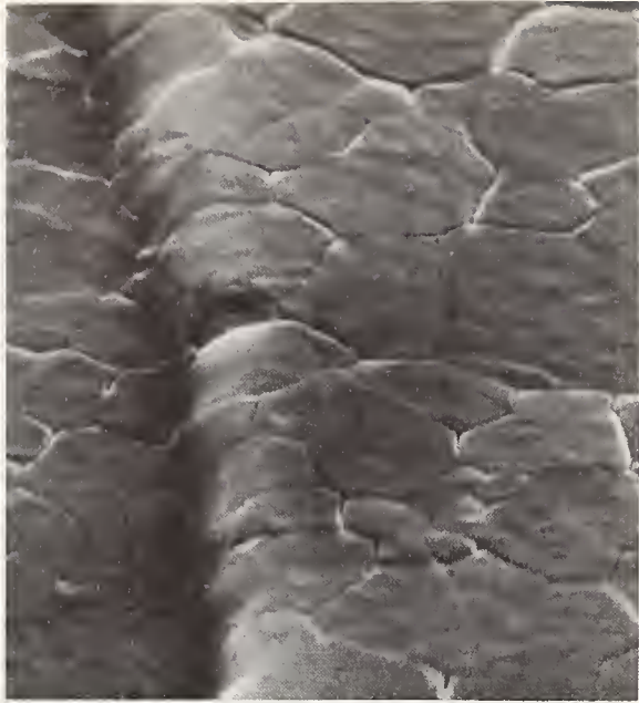
Fig. 4. Good Metal Step Coverage.
