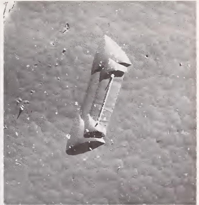
Fig. D.5. Replication micrograph showing a linear stacking fault terminated by two dislocation-etch pits.
