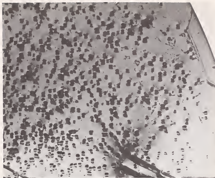
Fig. E.4. Example of contrast lobes due to poor adhesion between metal and \text{SiO}_2 .
