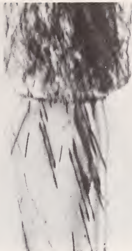
Fig. 9. Topograph of crystal section showing dislocations propagating from seed into body of crystal.
