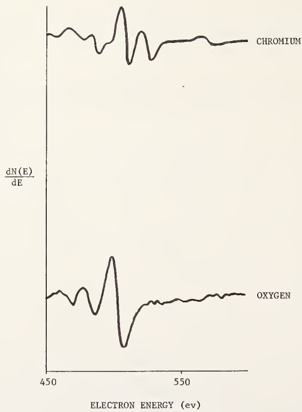
Figure 8 Auger Spectra of Chromium and Oxygen
