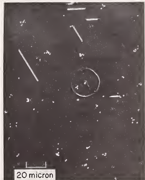
Fig. 7. Etch figures produced by a 2-minute Dash etch on a sample in which the oxygen was precipitated by annealing at 1100\text{ }^{\circ}\text{C} for 50 hours. Resistivity was 11.8\Omega\text{cm} ; boron doped; initial oxygen concentration of 12.9 \times 10^{17} atoms/cc.
