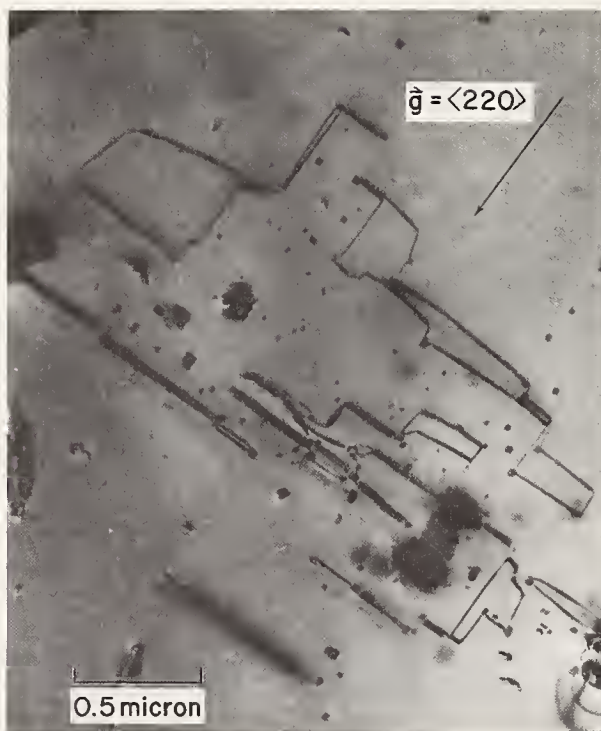
Fig. 3. TEM photo of typical defects appearing upon precipitation of dissolved oxygen. Plane of the sample is (100). The small square or rectangular contrasts arise from particles too small to be resolved.
