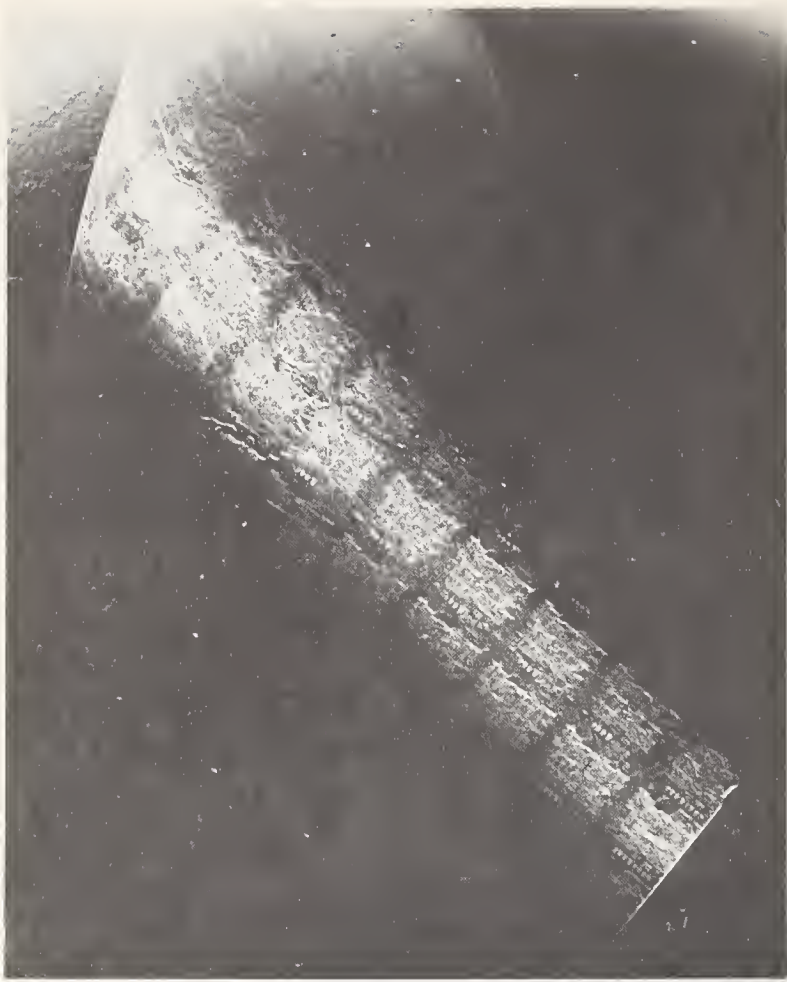
Fig. 11. Topograph showing high density of slip dislocations after base diffusion. Back surface mechanically-chemically polished.
