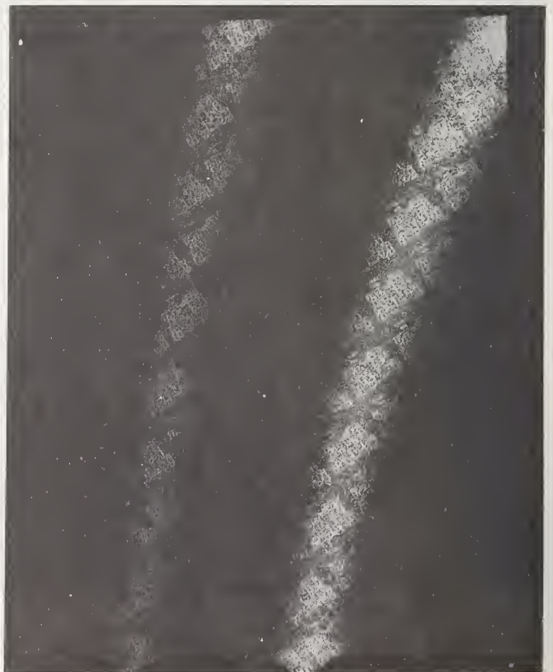
Fig. 12. A bent wafer with radius of curvature of about 500 cm. Back surface lapped.
