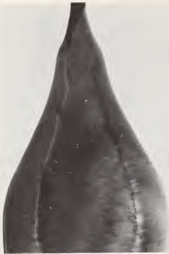
Fig. 12. Topograph of crystal section showing dislocations propagating from seed into body of crystal.
