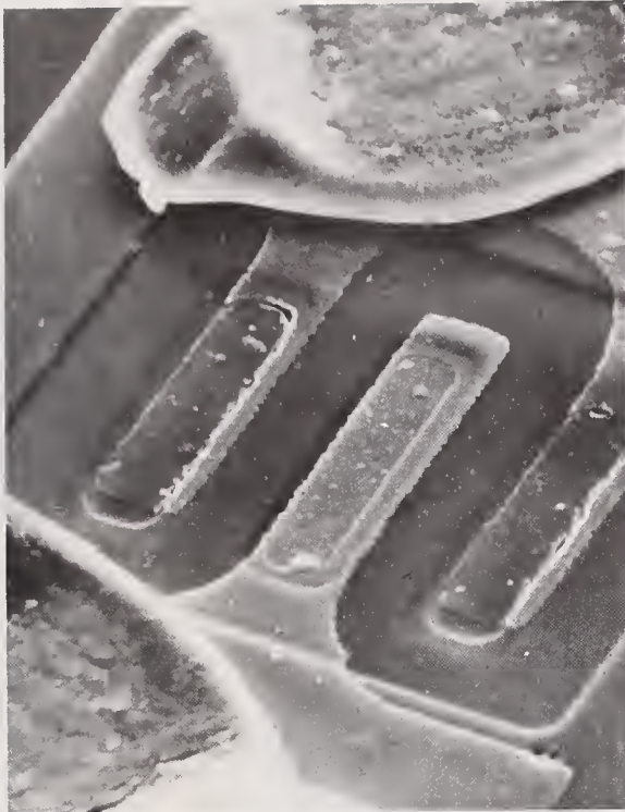
Fig. 1. Transistor with Base Metal Step Defects.
