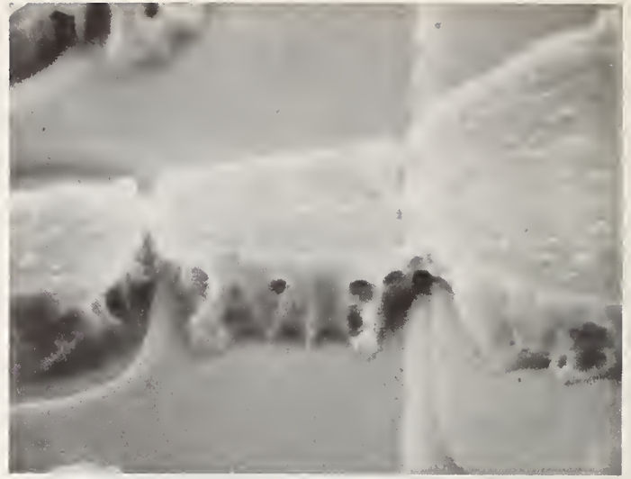
Fig. 5. Damage Due to Etchant Entering Step Defect.
