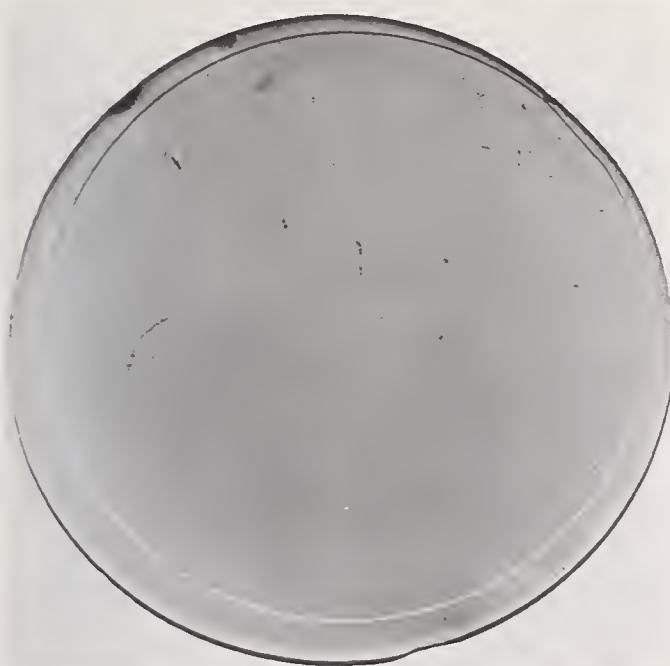
Fig. E.5. SOT topograph of oxidized Si sample after Al evaporation (circular region 0); the lack of contrast lobes in the film region indicates good adhesion.
