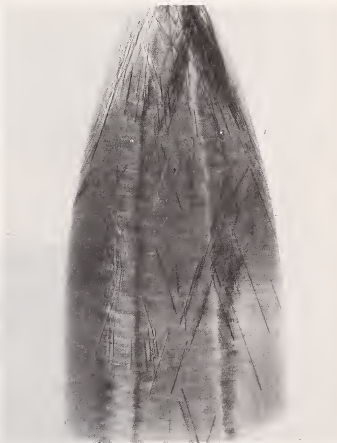
Fig. 11. Topograph of crystal section showing dislocations propagating from seed into body of crystal.
