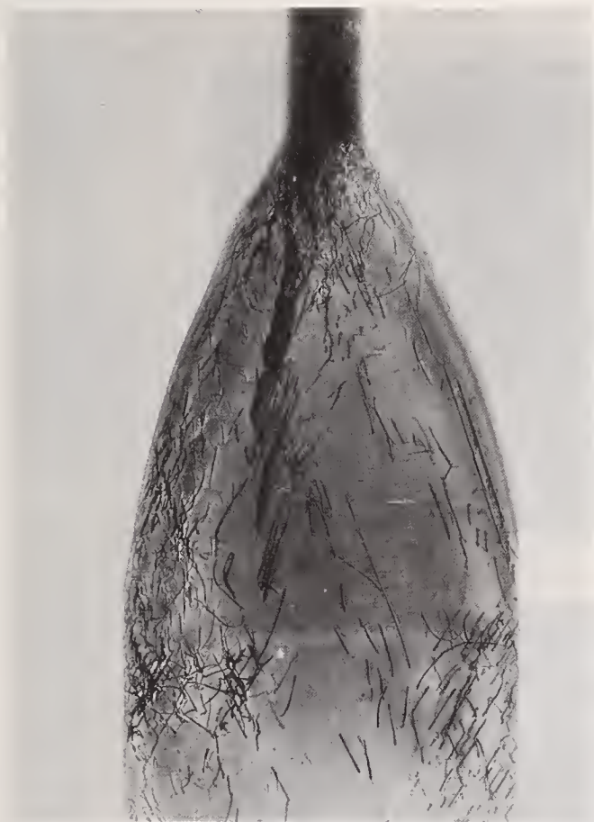
Fig. 10. Topograph of crystal section showing dislocations propagating from seed into body of crystal.
