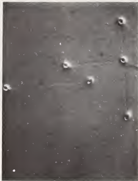
Fig. 7(a) - Differential interference micrograph of mechanically polished silicon surface after stripping 0.8\mu\text{m} of 1100^\circ\text{C} dry oxygen grown oxide and Sirtl etching. 360\times
