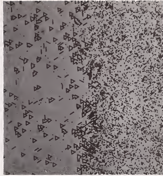
Fig. D.3b. Relative difference in dislocation density is revealed after a 1-min Sirtl etch.
