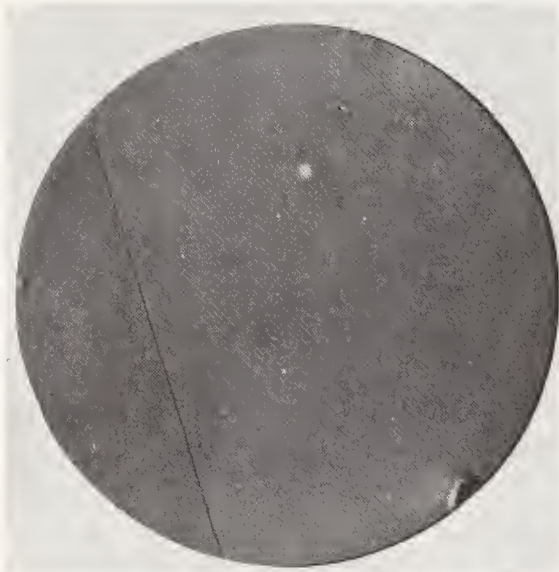
Fig. D.2a. SOT topograph of damage contrast due to mechanical polishing
