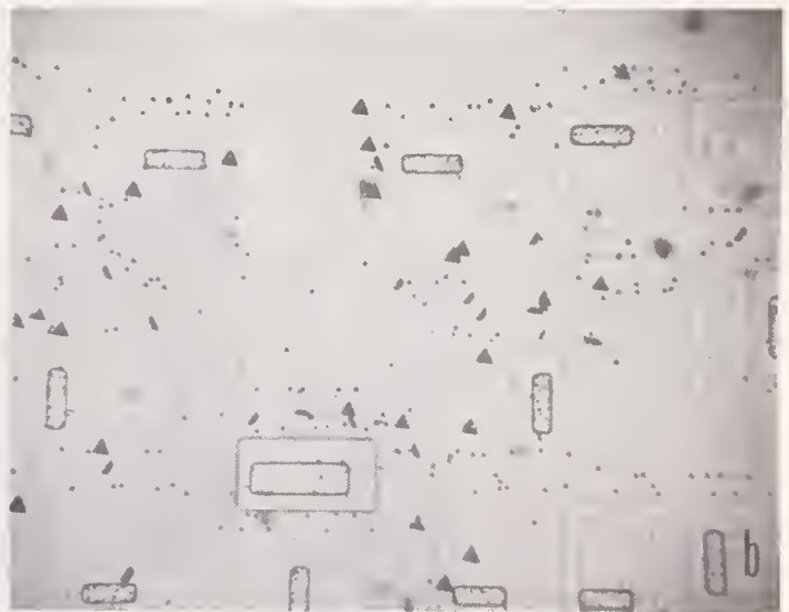
(b) Stacking faults due to poor cleaning of the wafer before epitaxial deposition.
