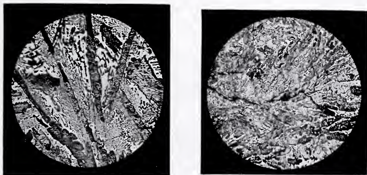
Figure 1. Comparison of Structure From Different Regions of a Copper Alloy (Microscopic). Illustrating article "Photography in Research and Science," by Arthur G. Eldridge.
