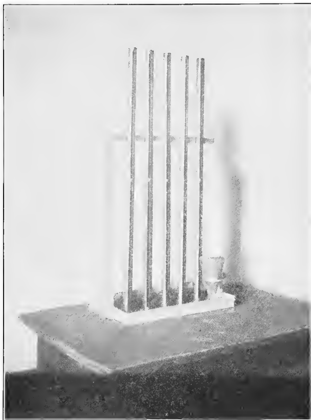
APPARATUS USED TO COMPARE THE CAPILLARY RISE OF MOISTURE IN DIFFERENT SOILS
