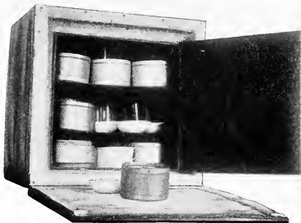
DOUBLE-WALLED DRYING OVEN HEATED BY TWO ELECTRIC-LIGHT BULBS
