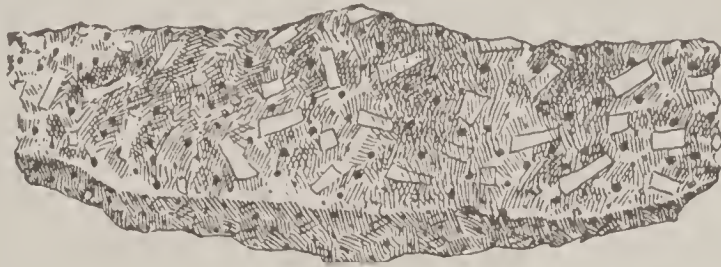
Granite with black mica and feldspar crystals, with quartz as chief base.
