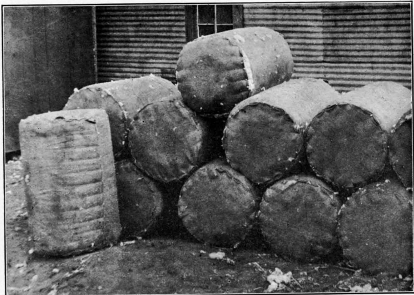
FIG. 1.—THE ROUND COTTON BALE, WHICH IS PUT UP AT THE GIN WITH A DENSITY GREATER THAN THAT OF THE COMPRESSED BALE. IT IS ABOUT 3 FEET LONG BY 20 INCHES IN DIAMETER, WEIGHS ABOUT 250 POUNDS, CARRIES 1 PER CENT TARE, AND CAN BE SHIPPED DIRECT FROM GINNERY TO MILL.
