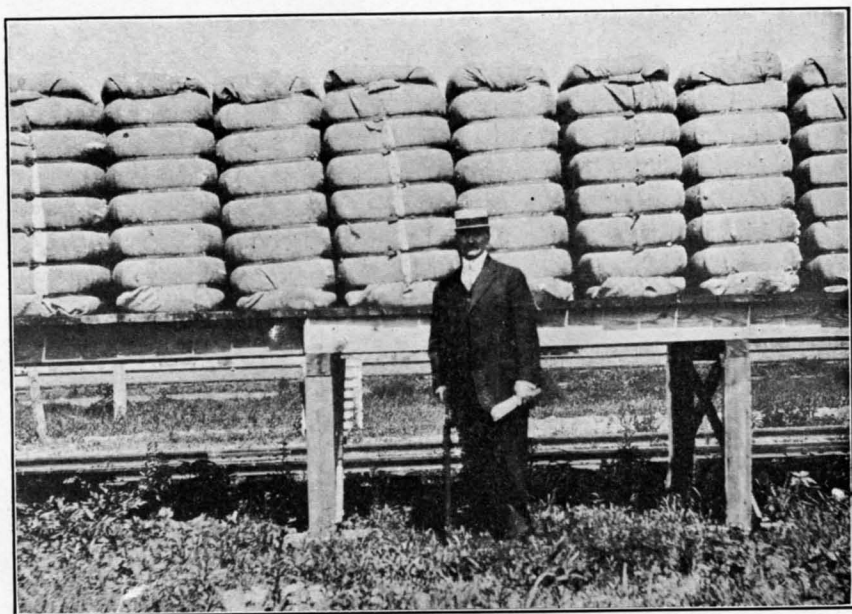
FIG. 2.—GIN-COMPRESSED SQUARE COTTON BALES, COMPLETELY COVERED, HAVING A GREATER DENSITY THAN ORDINARY COMPRESSED BALES AND CARRYING LESS THAN HALF THE TARE. THOSE SHOWN ARE FOR SHIPMENT DIRECT FROM GIN PLATFORM TO BREMEN, GERMANY.
