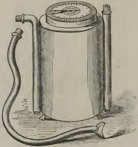
A spirometer, made upon the plan of the dry gas meter, has been for some time employed in Germany, and was introduced into use in this country by Dr. S. Weir Mitchell. It is altogether more simple in its management than the rather clumsy instrument of Hutchinson, and affords fully as accurate results. (Fig. 3.)
