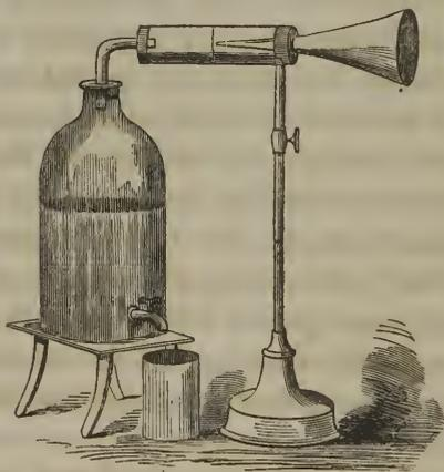
the pointed extremity of a small copper funnel, the other was connected with an aspirator. The apparatus is shown in the accompanying cut. (Fig. 11.) Into the large tube a
