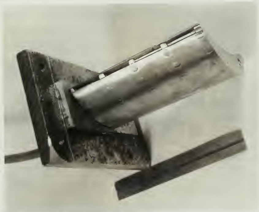
FIG. 14 HORIZONTALLY GROOVED AIR COOLED TURBINE BLADE MODEL WITH COVERING METAL SLEEVE
