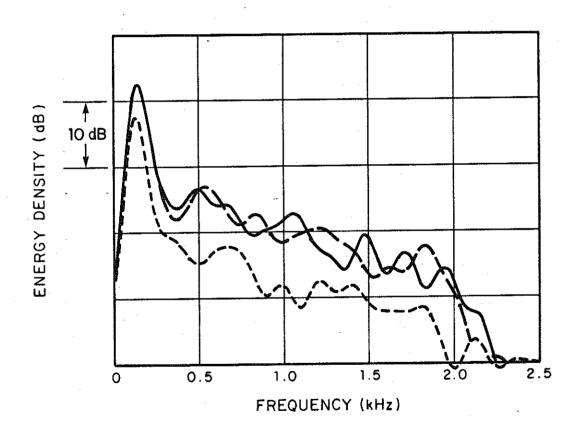
Fig. 4: Energy Spectra of Shots No. 28 and 29 on Compensated WKYC-TV Recording
