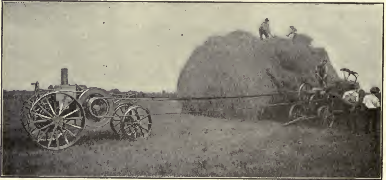
FIG. 202.—Hay-baling machine driven by traction engine.
