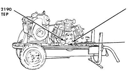
MODEL LP-512 ENG-2 MODEL LP-832-ENG-2 Air Compressor Crankcase Oil Level Sight Gage (Check level)
