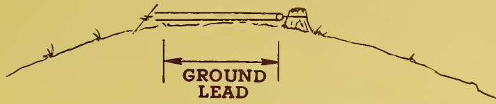
Figure 7.—Ground lead condition on crest of ridge.
