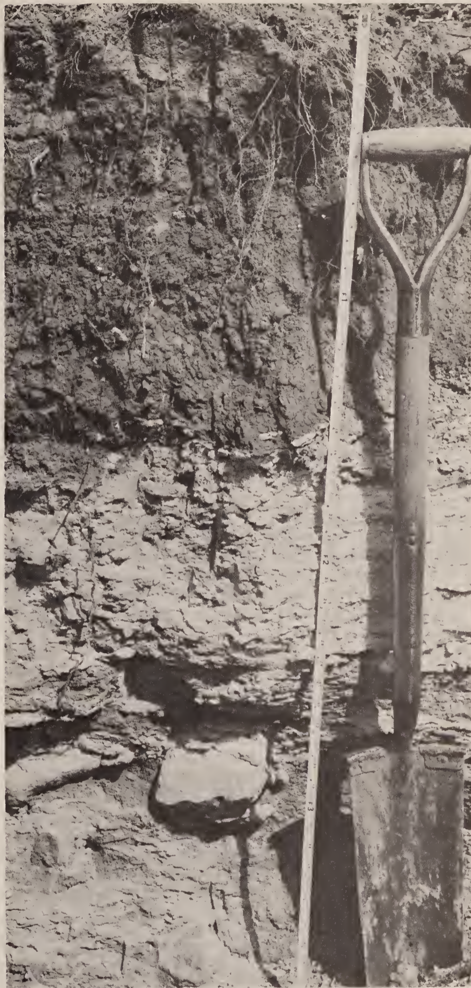
Figure 10.—Pavant loam, 4 to 8 percent slopes. The indurated hardpan is at a depth of about 17 inches.
