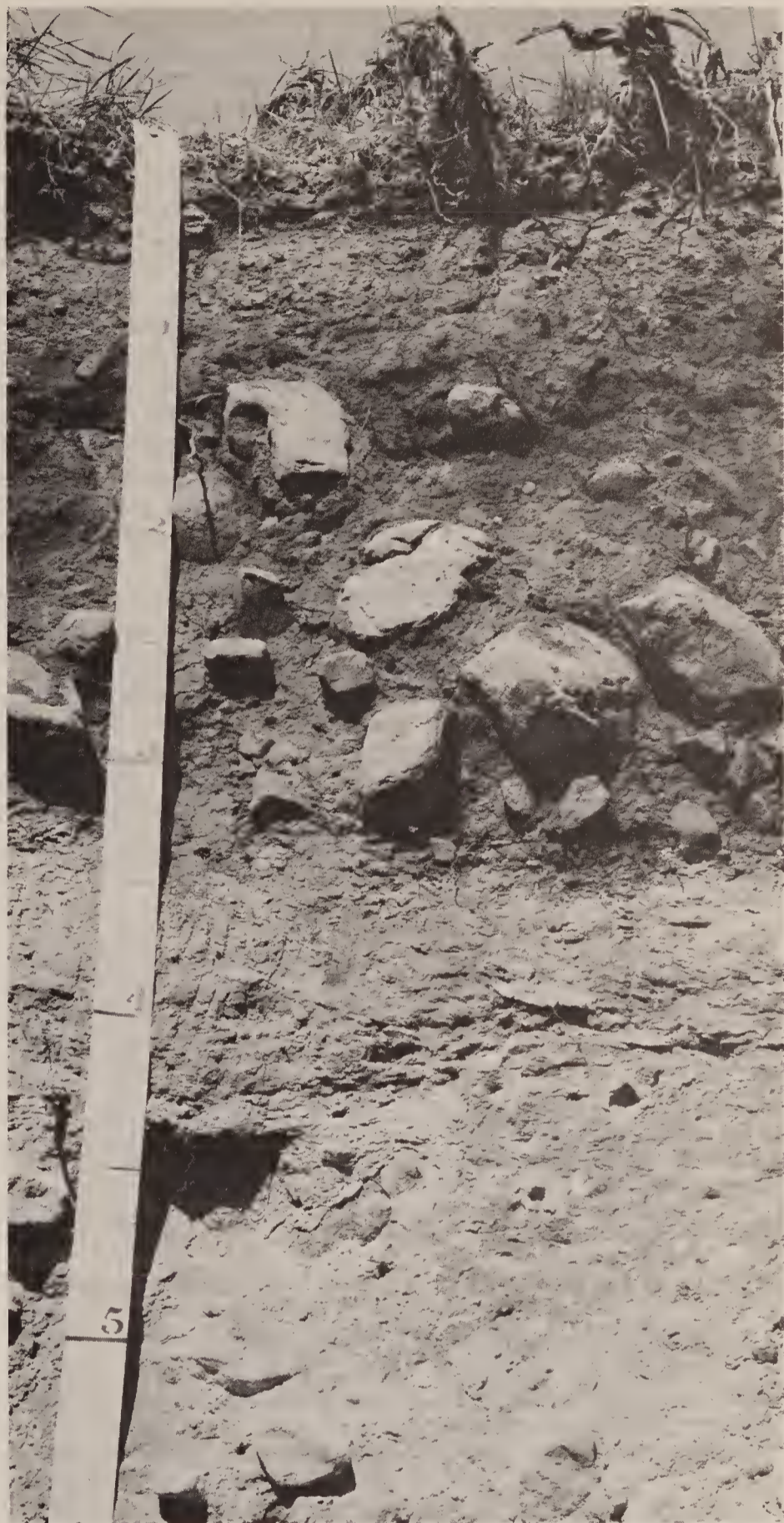
Figure 9.—Mountainville very stony sandy loam, 2 to 8 percent slopes. Depth is marked in feet.
