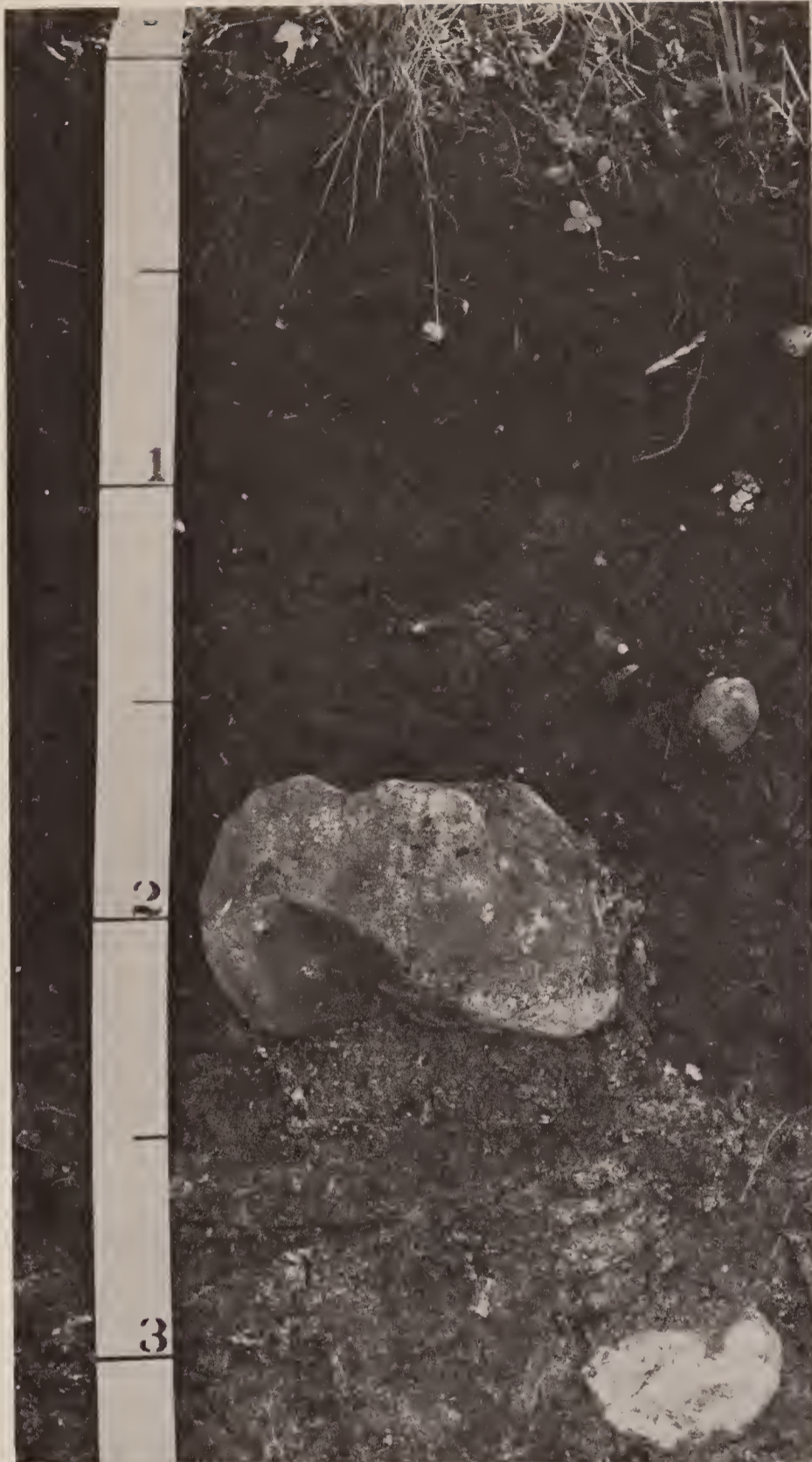
Figure 5.—Deer Creek stony silt loam. The light-colored underlying layer contains accumulated lime. Depth is marked in feet.
