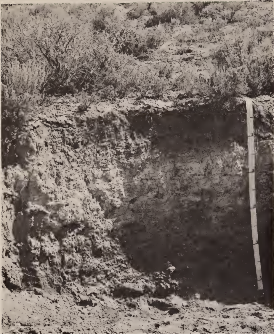
Figure 1.—Arapien fine sandy loam, 2 to 5 percent slopes, eroded. A light colored, limy layer is between depths of 10 and 38 inches.
