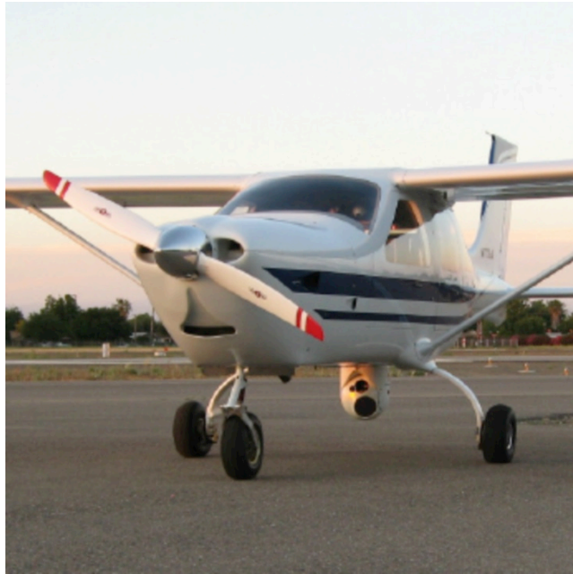
Figure 14. Multi-Mission LLC, Multi-Mission Aircraft (MMA) with WESCAM MX-15 Gimbal with Electro-optical and Infra-Red Cameras 38
