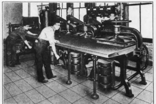
ELECTRIC PNEUMATIC MATRIX DRYING TABLES USED IN PLANT OF BROOKLYN EAGLE
