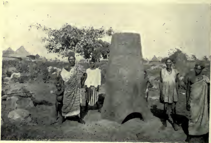
COURT OF THE KING OF BANGJELI, IRON SMELTER. THE ORES DUG AND SMELTED BY THE NATIVES CONTAIN ABOUT 50 PER CENT. OF IRON.
