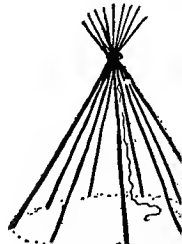
2 nd Set up 6 poles
