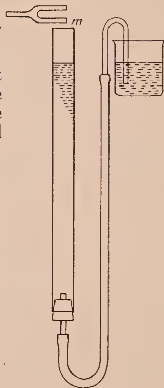
Fig. 22. Vertical form of resonance tube. The length is adjusted by raising and lowering the water.
