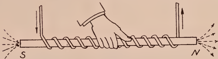
Fig. 31. The right hand rule for a coil.
