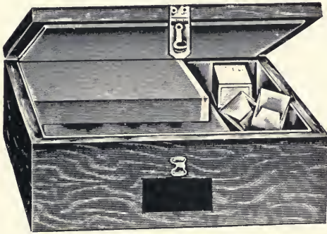
Fig. 60.—X-rayproof film and plate chest.
