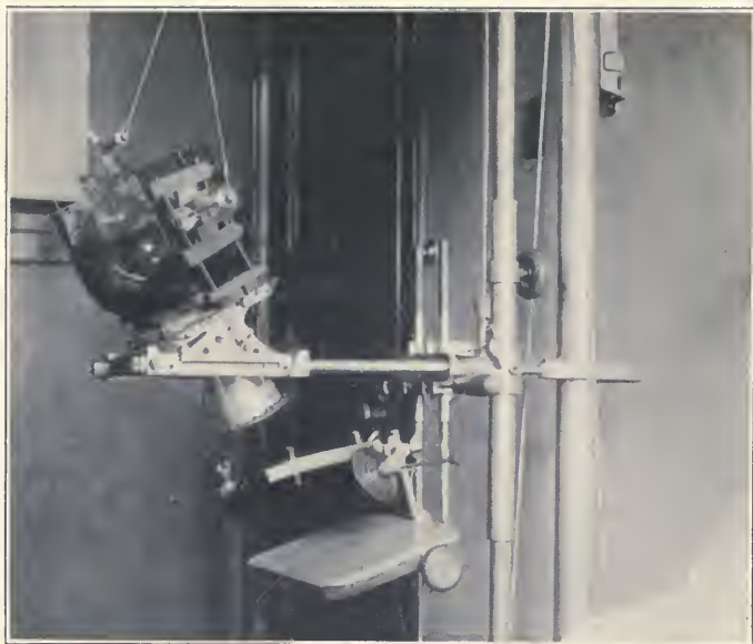
Fig. 43-A.—Tube stand with platerest and head support. (Eisen and Ivy.)
