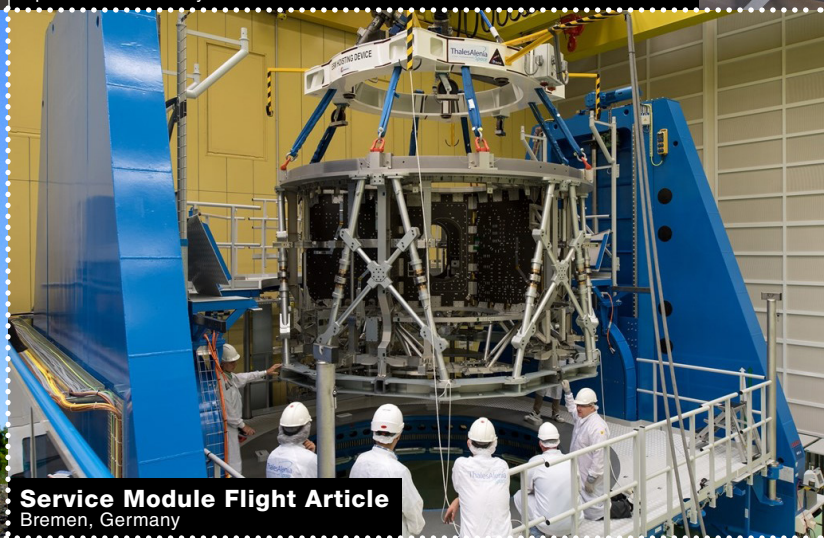
Service Module Structural Testing Space Power Facility at NASA Glenn Research Center's Plum Brook Station
