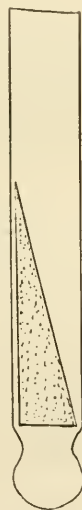
FIG. 211.—Culture tube with bulb to hold glycerine and water below slant of vegetable.
