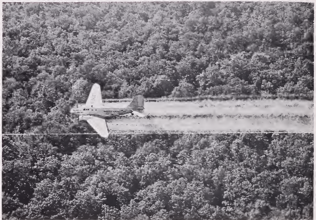
*BN-4082--Multi-engined planes disperse a spray of DDT-oil solution over areas infested by the tree-attacking gypsy moth. The insecticide remains effective for at least 3 weeks. Applied at the rate of 1 pound of DDT in one gallon of oil per acre, it is harmless to humans and does no damage to wildlife.
