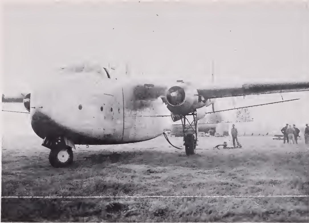
*BN-4083--Planes are being loaded here with DDT insecticide in oil solution from large tanks seen in the background. Planes and pilots are subject to Civil Aeronautics regulations. Before each take off pilots and copilots are carefully briefed on areas to be sprayed and pattern to be followed. Spraying is done in early morning hours when air is still.
