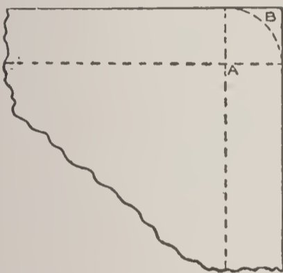
Fig. 57. Marking Off Bottom Sheet of Lead for Tank Lining. Leaving Edge to be Turned Up.
