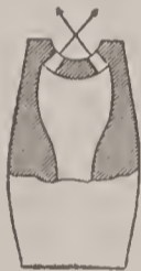
Fig. 108. Vertical Section of Union-Jet Burner.
