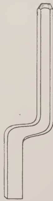
Fig. 250. Right and Left "Corner" Tools for Calking and Yarning.
