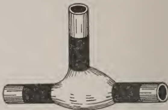
Fig. 243. Combination Branch and Round Joint.
