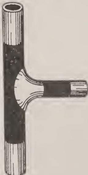
Fig. 238. Branch Joint with Concave Neck.
