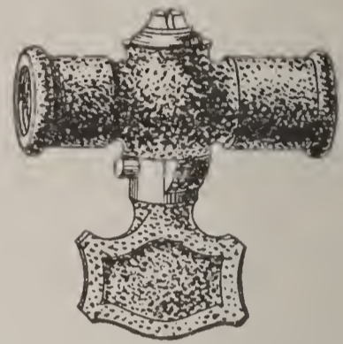
Fig. 115. Single Gas-Cock with Stop-Pin.
