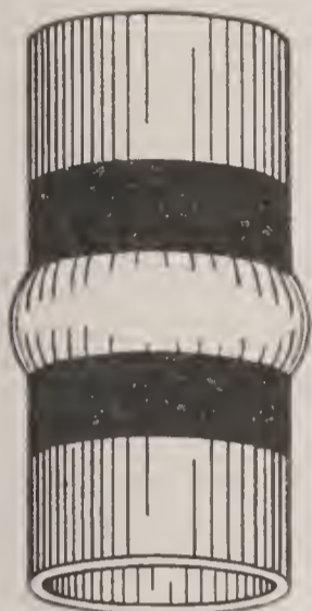
Fig. 237. Round Joint on Large Pipe.
