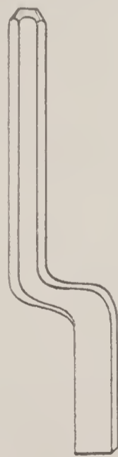
Fig. 250. Right and Left "Corner" Tools for Calking and Yarning.
