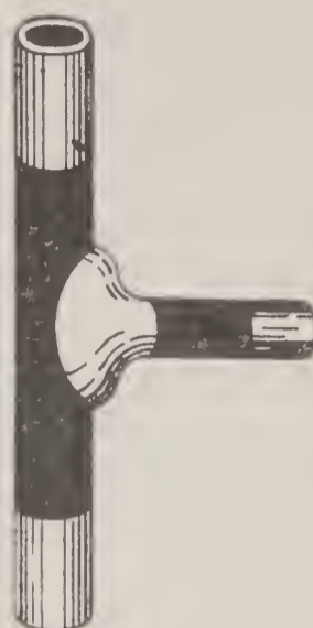
Fig. 239. Branch Joint with Swell Neck.
