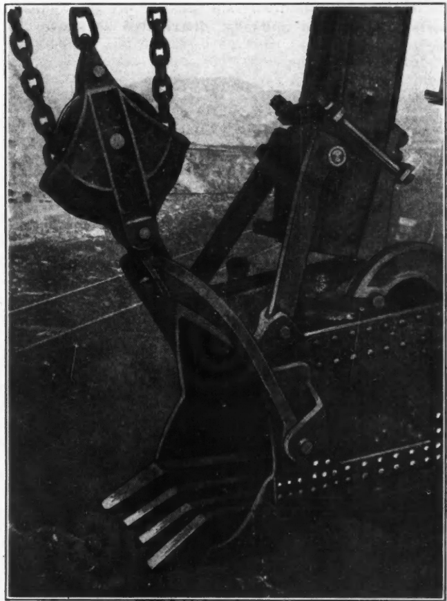
DIPPER BOOM REPAIRED BY MEANS OF YOKE
