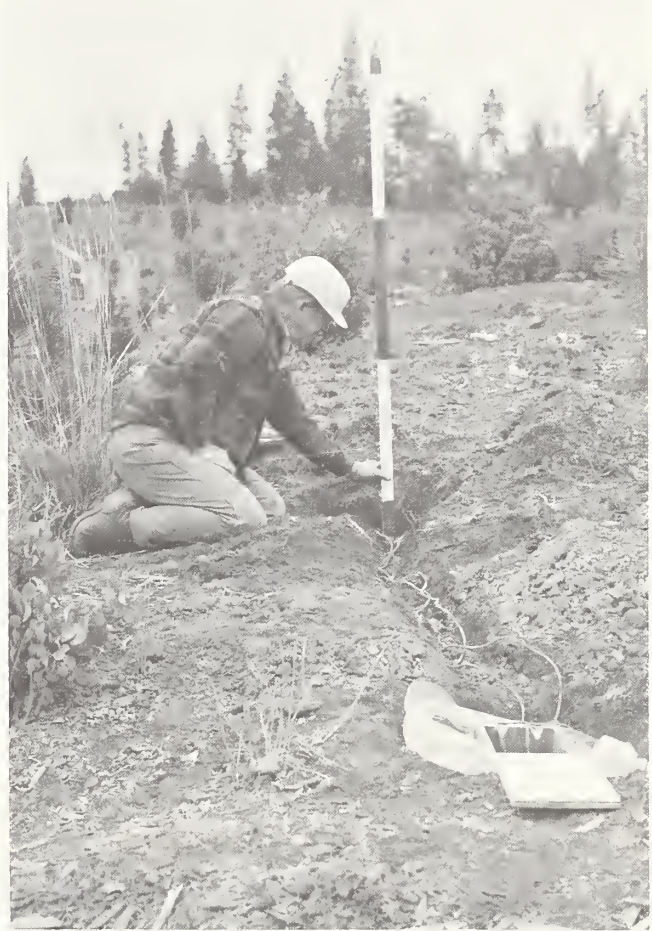
In a study of mineral cycling and fertilization in a mixed-conifer plantation, soil temperatures are monitored through probes.
