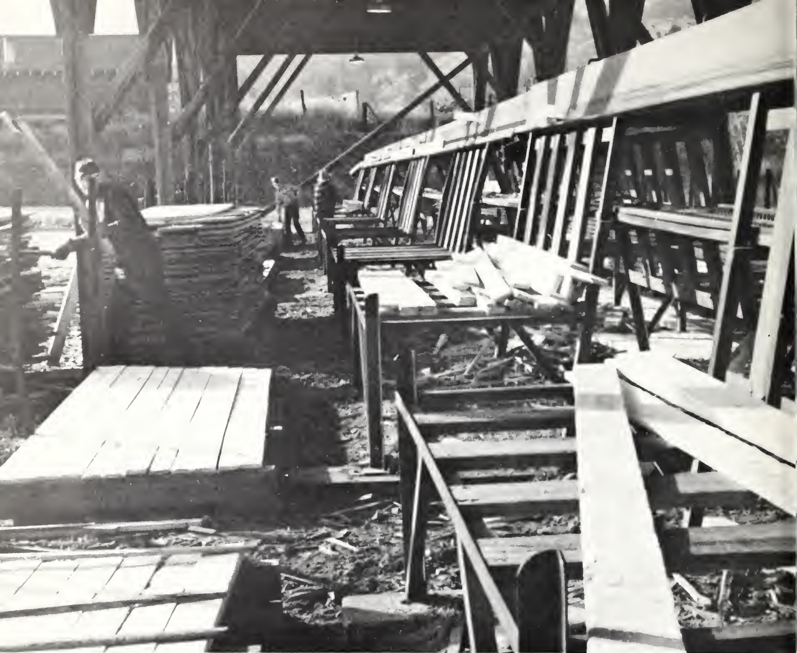
Lumber of several dimensions and grades, cut from study trees at a cooperating sawmill, is sorted for drying.
