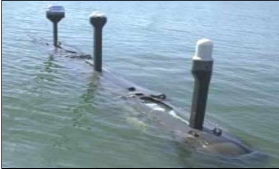
Figure 13. Monopole retractable antenna concept as used in the Sea Stalker UUV (From: Mullins, 2009)
