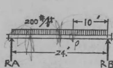
$$\begin{aligned} M_{\max} &= \frac{w \cdot l^2}{8} = \frac{200 \times 24^2}{8} \\ &= 14400 \text{ 呎封度} \\ &= 14400 \times 12 \\ &= 172800 \text{ 吋封度} \end{aligned}$$
