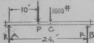
$$M_{max.} = M_C = \frac{W \cdot l}{4} \\ = \frac{1000 \times 24}{4} = 6000 \text{ 呎封度} \\ = 6000 \times 12 = 72000 \text{ 吋封度}$$
