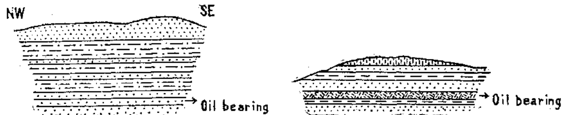
Fig. 5. Section showing the oil-bearing horizon (fine grained sandstone) on the NW of Huchlachuan, Yench'anghsien.
