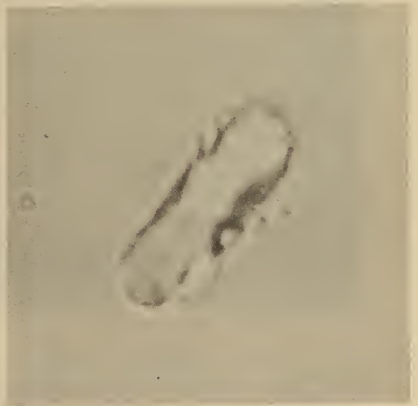
Figure 3. Sheaflike appearance which is characteristically seen when an aggregate of the type shown in figure 2 is rotated through 90^\circ about any axis in the plane of the microscope stage. (Unpolarized light x 2000).
