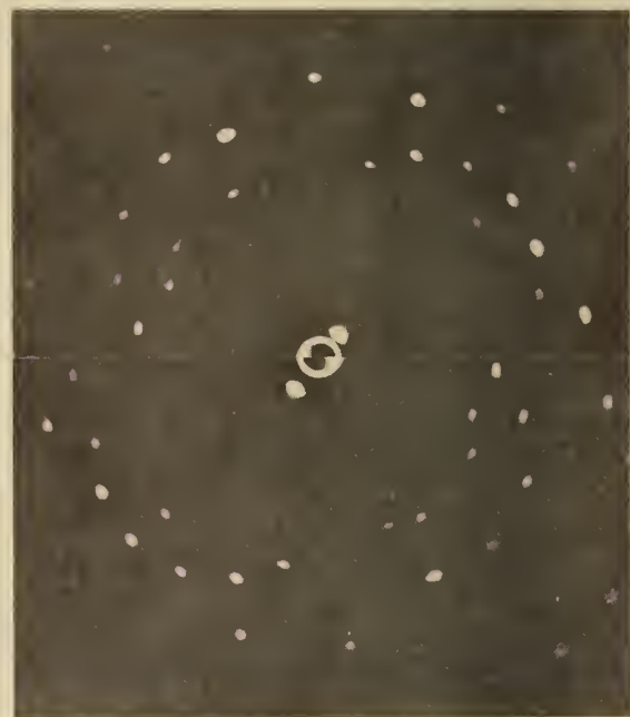
Figure 15. Two half Laue diagrams of ammonium dihydrogen phosphate crystals grown respectively top with and bottom without addition of \text{Cr}^{3+} ions. Corresponding Laue spots are diagonally opposite each other.
