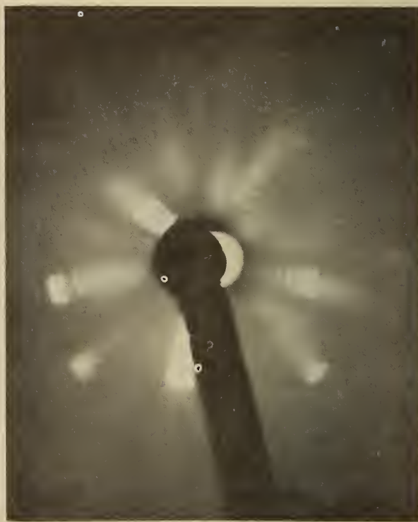
Figure 13. Laue diagram of potassium crystal showing much orientation spread.
