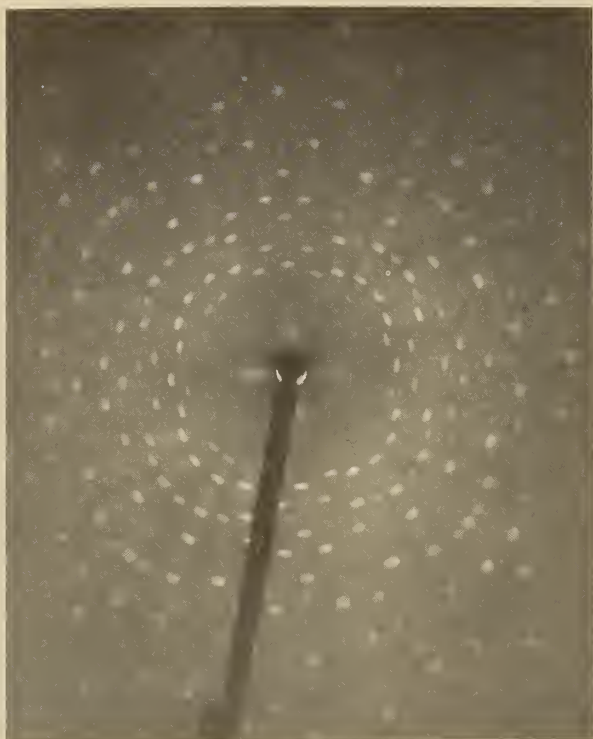
Figure 12. Laue diagram of a \sim 3 -mm thick ammonium dihydrogen phosphate crystal section perpendicular to the fourfold axis
