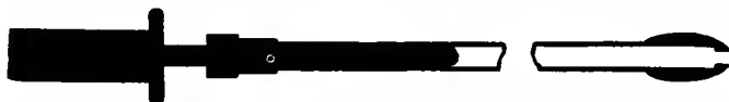
Fig. 25. The King soil tube, used for collecting samples of soil. The heavy hammer is used to drive the brass tube into the soil, while the cutting edge with the small diameter cuts out a core of soil which slides readily up into the tube.
