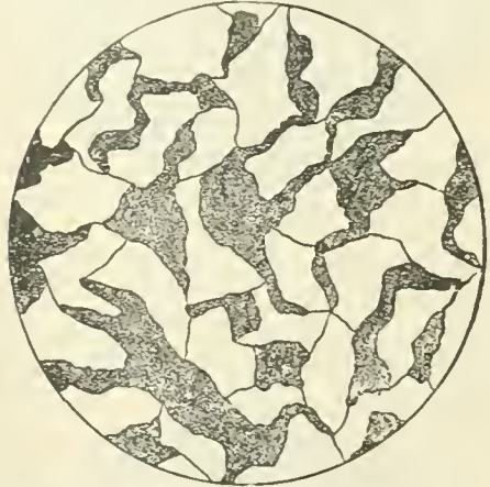
FIG. 7.—Structure of Medium High Carbon Steel. Carbon 0.38 per cent (Arnold) Ferrite and Pearlite.
