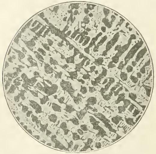
FIG. 12.—Structure of White Cast Iron Magnified 150 Diameters (Longmuir). Pearlite and Cementite.
