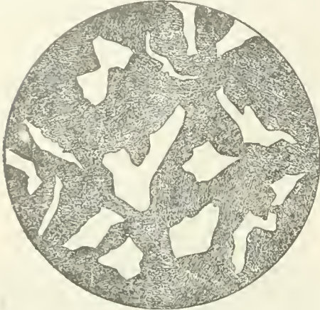
FIG. 8.—Structure of Medium High Carbon Steel. Carbon 0.59 per cent (Arnold) Ferrite and Pearlite.
