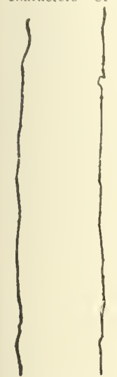
FIG. 4.—A tracing by camera lucida of the margins of an ink line drawn by a pen fixed to a ruling machine. It is enlarged 60 diameters. There is an absence of the irregularities always found in the margins of ink lines made by the human hand.
