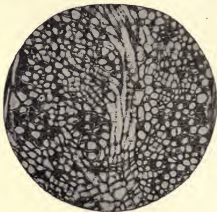
FIG. 127.—Portion of large ray highly magnified, showing presence of tracheary elements in ray substance.
