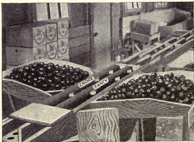
Upper end of the machine with bins of apples on each side. The sorters work at these bins.
