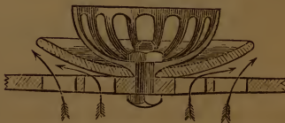
MAUDSLAY'S DISC VALVE FOR AIR PUMP. Section.
