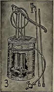
Fig. 8. BONANZA D. A. SPRAY PUMP. The best spray pump of large capacity made. Brass ball valves and guided piston rod. Fitted with 8 ft. 1 1/4 in. wire-lined suction hose, two Y connections for hose. One, two, three or four lines can be used. Hose nozzles and extension pipes additional. As shown in cut, Fig. 8. . . . . Our net price 30.00
