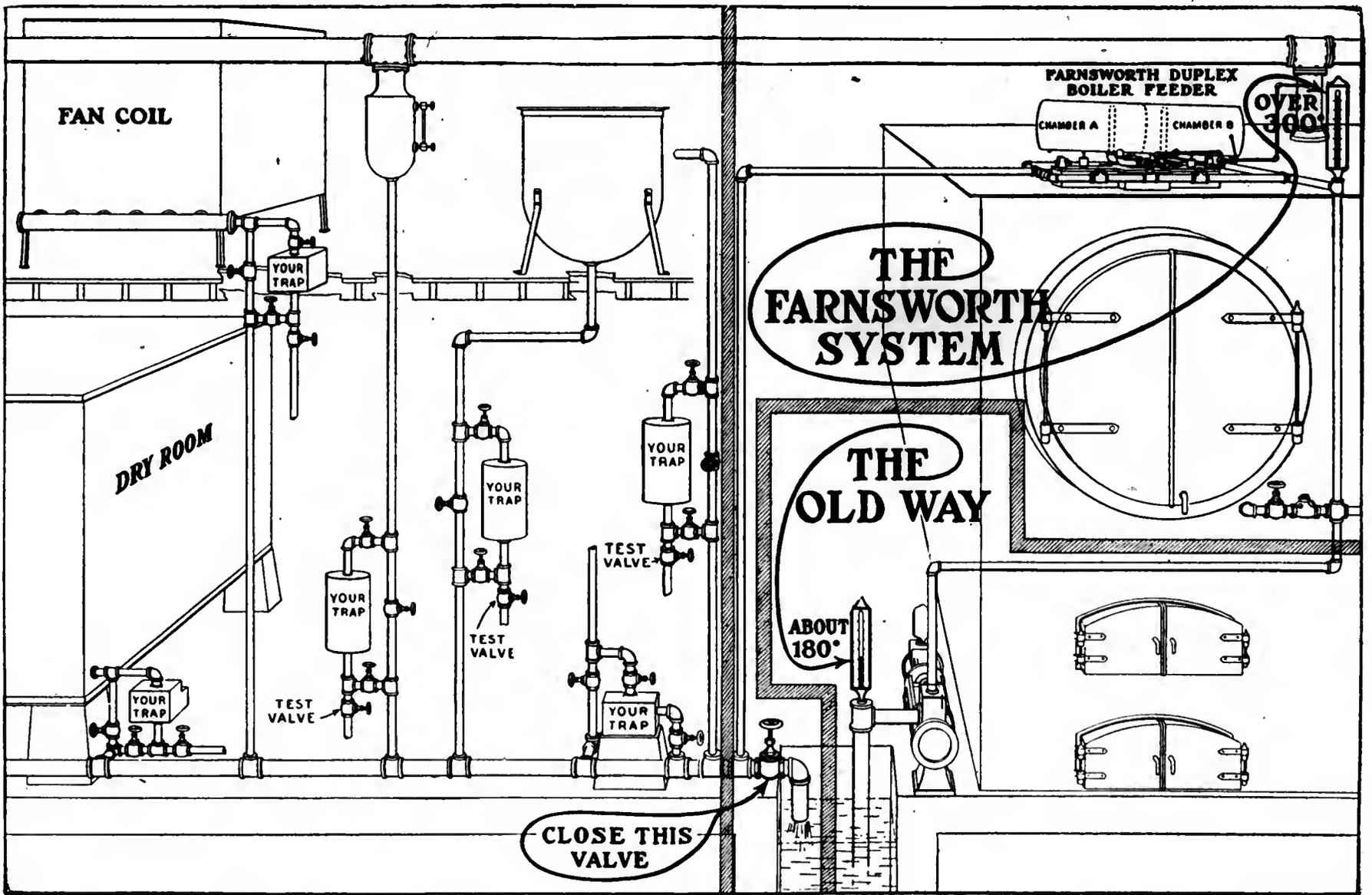
Place the Farnsworth Duplex Boiler Feeder above your boilers — discharge all your high pressure traps directly into it. Any L. P. condensation you have in scattered buildings drain to a Farnsworth Condensation pump, which will pump it to this Duplex Boiler Feeder. By this closed system all condensation is held under pressure and fed directly into boilers at a high temperature.
