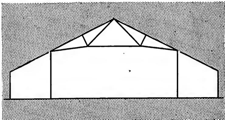
So [scientifically framed is that part of our house included between the two columns, that it would stand staunch and firm entirely independent of the side posts. The part from the side posts to the column is really a lean-to. This being so, the needlessness of a post heavier than we use is apparent.
