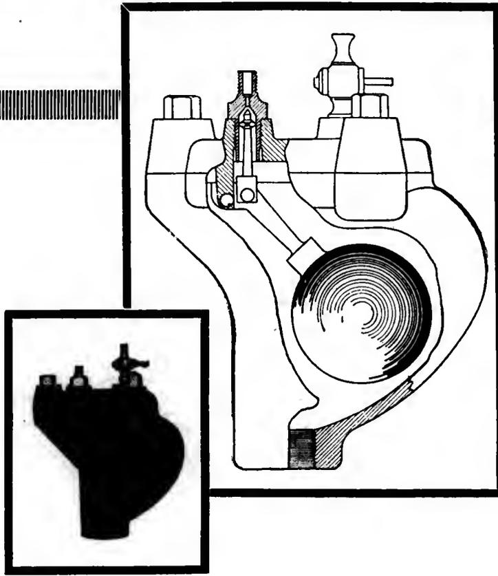
Cross Section View of Fisher Air Trap Type 30, showing how air is relieved.
