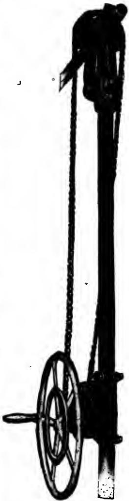
Note machine operates on worm and gear principle. All gears are entirely enclosed so that no water or dirt can get onto them.
