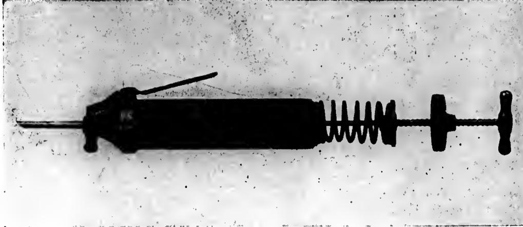
The *spring* does the work. It forces the material from the machine in a steady flow. Press the lever and the machine does the rest. **Use ONE HAND only when using the Vita Automatic Machine.**
