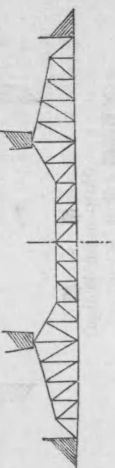
懸木橋 (Cantilever bridge)
