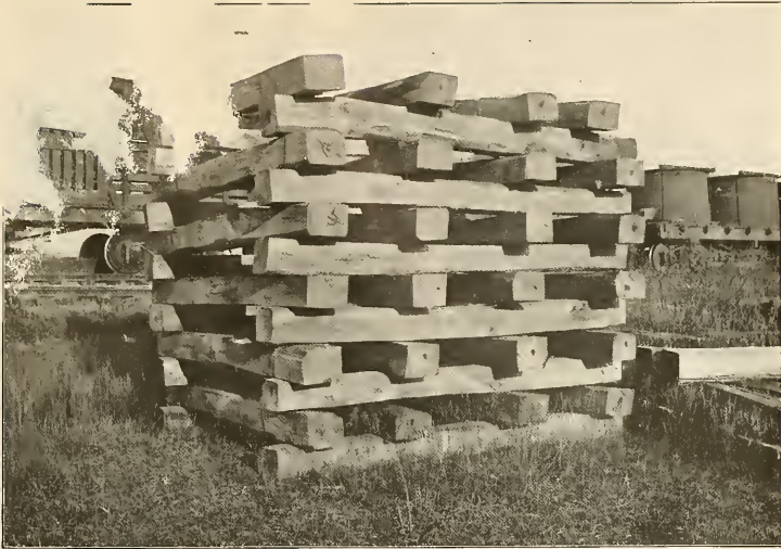
FIG. 1.—OPEN-CRIB OAK PILE, SOUTHERN ILLINOIS.
