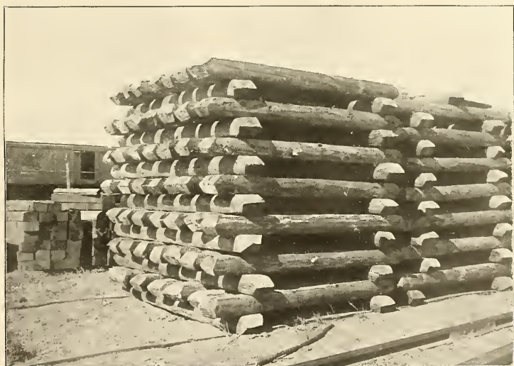
FIG. 2.—AFTER TREATMENT. LOGGEPOLK PINE, OPEN-CRIB PILE.
