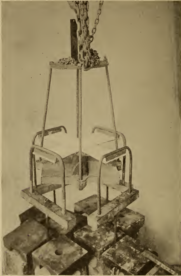
FIG. 5. VIEW SHOWING CROSS-BENDING TEST SPECIMEN UNDER LOAD.
