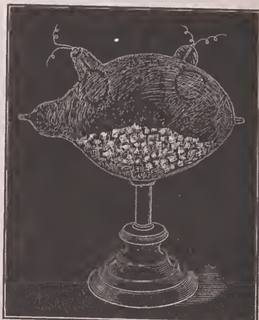
FIG. 4.—A Crookes tube showing luminescence of crystals under action of cathode rays.
