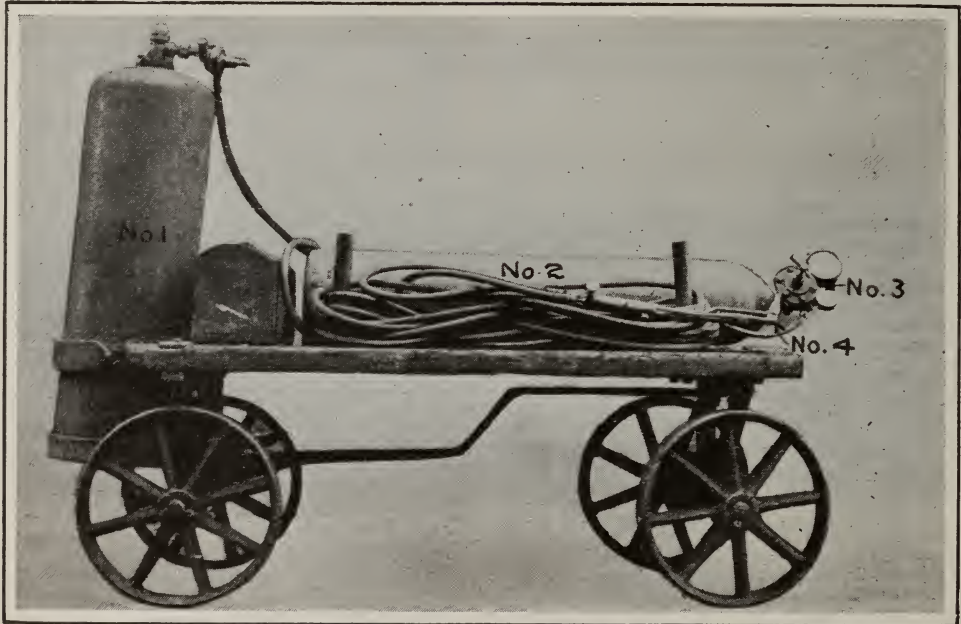
THE OXY ACETYLENE EQUIPMENT NOW IN USE
