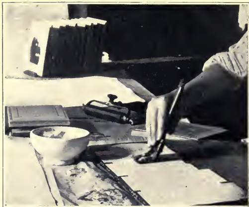
Illustration No. 57 Applying Paste to Back of Print See Paragraph No. 468
