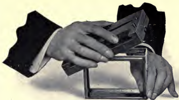
Illustration No. 39. Attaching Loading Block to Plate Rack. See Paragraph No. 33I.
