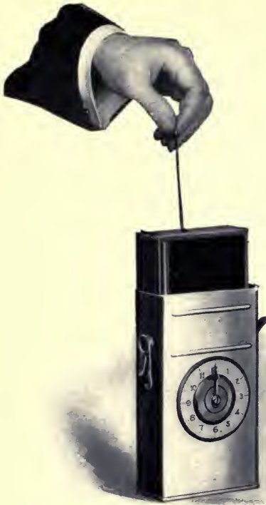
Illustration No. 41. Lowering Rock of Plates Into Solution Cup. See Paragraph No. 331.
