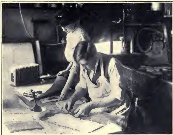
Illustration No. 58 Method of Picking Up Prints after Applying Paste See Paragraph No. 468
