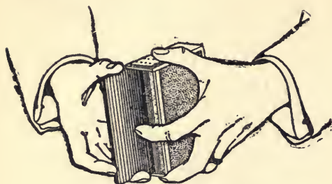
Illustration No. 43. Removing Plates from Rack. See Paragraph No. 335.
