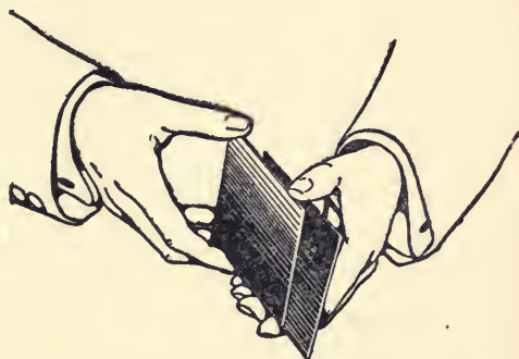
Illustration No. 44. Separating Plates after Removal from Rack. See Paragraph No. 335.
