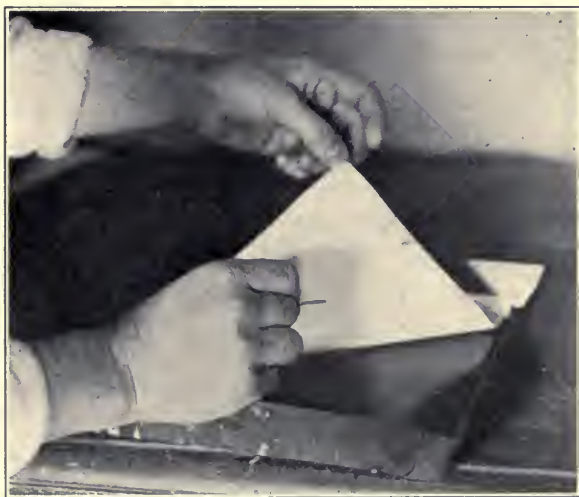
Illustration No. 53 Sensitizing the Paper—Removing Air-bells See Paragraph No. 370
