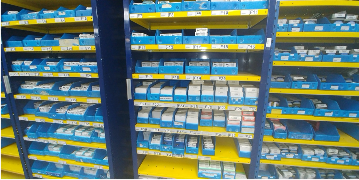
Figure 4. NOSTRA's Two-Bin Kanban Shelving System. Source: E. B. Walters (personal communications, April 22, 2019).
