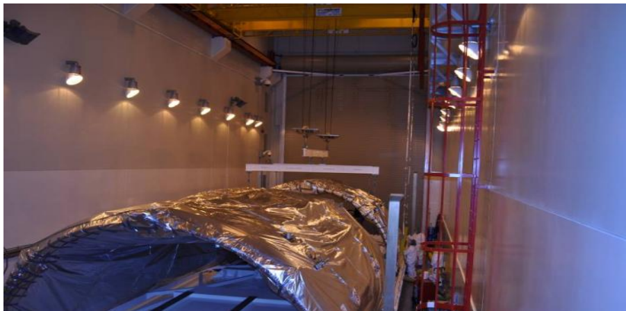
Figure 15. Payload Fairing Inside of IPF near SLC-6
