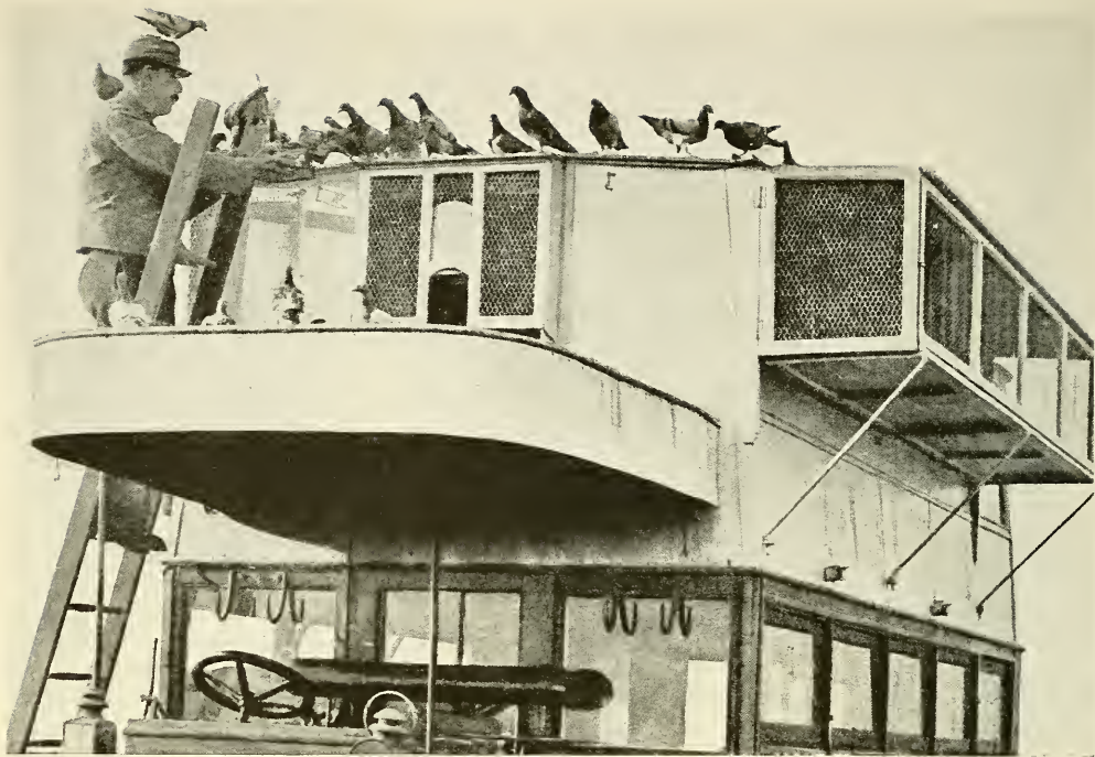
MESSENGERS OF THE AIR: THE FRENCH ARMY AUTO AT THE FRONT FOR CARRIER-PIGEONS
