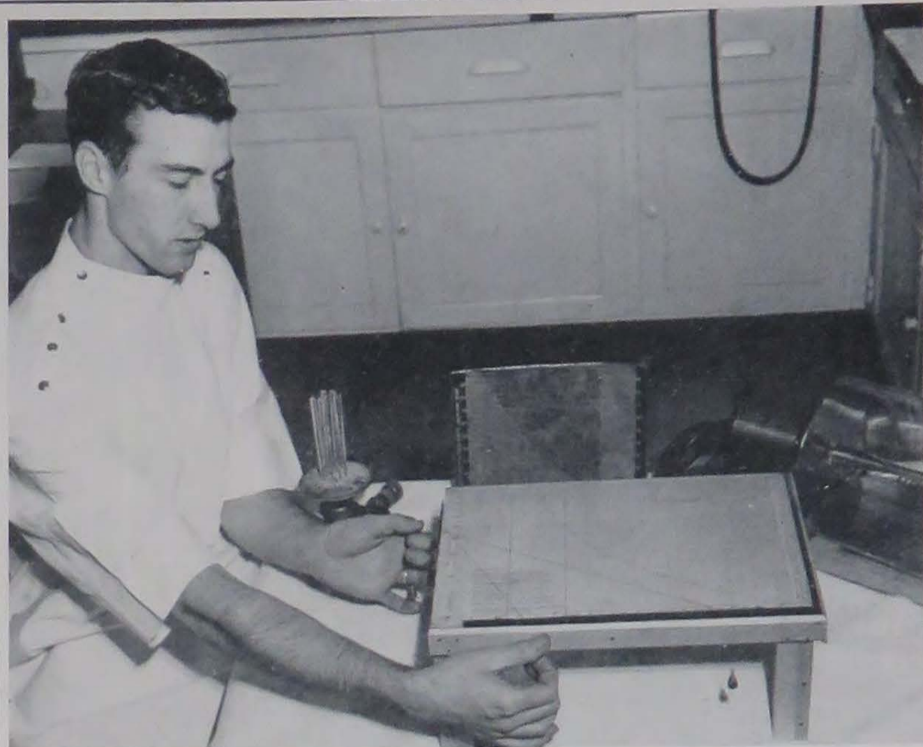
Tom Durkee, HM3, student-inventor of the Laboratory Technician's School, is shown demonstrating how his latest invention—a "protein-bound iodine calculator"—works, by means of threads, with weights on either end, placed over a graph, eliminating the work of measuring and drawing lines on a similar graph. Also on the table are several of his other "gadgets" that are now in use in the hospital's laboratories.
