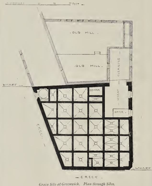
Grain Silo at Greenwich. Plan through Silos.
