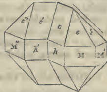
Compound crystal composed of three so united that their upper edges meet at angles of 120°.
