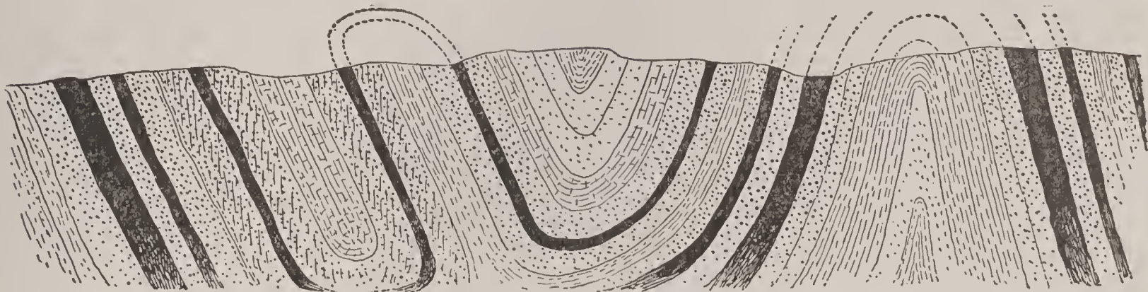
CROSS SECTION OF ANTHRACITE COAL MEASURES (PENNSYLVANIA).
