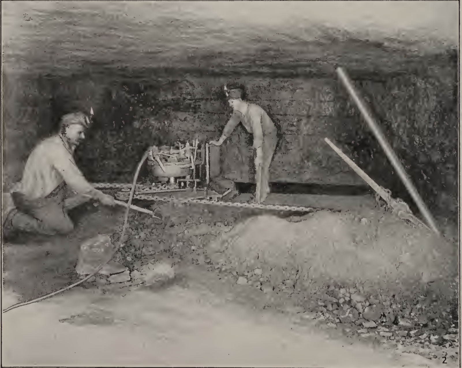
1. SULLIVAN ELECTRIC CHAIN MACHINE, Making "tight" or corner cut.
