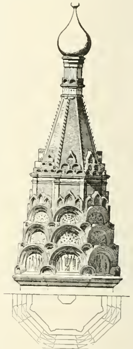
RUSSIA, FIG. 3: TOWER OF VASILII BLAJENOI, MOSCOW; RECEDED ARCHES DIMINISHING SIZE OF CENTRAL OPENING.
